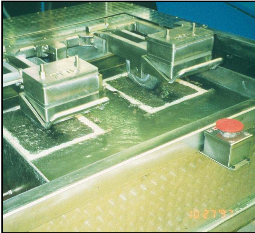
Figure 12. The Hamburg Wheel-Tracking Device (HWTd)
